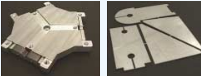
Above: A couple of typical parts. Notice secondary machining (Left), and tabs used to hold pieces (Right).
